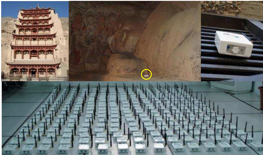
Fig. 2. Microclimate monitoring at Mogao Grottoes: [top left] a representative building, [top middle] a sensor deployed inside Cave C158, [top right] a sensor deployed at the cave entrance, [bottom] 300 sensor nodes.
