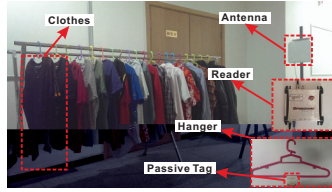
Fig. 10. Action recognition detection evaluation scene
